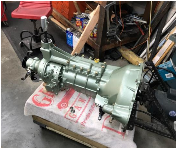
Details of the BJ8 Gearbox with Sebring ratio straight cut gears.
