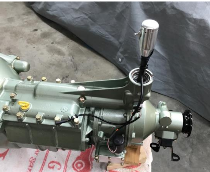
Details of the BJ8 Gearbox with Sebring ratio straight cut gears.
