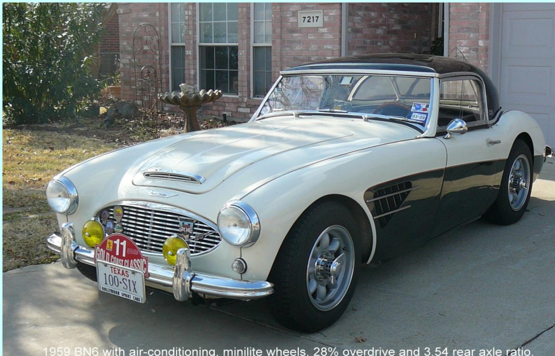
1959 BN6 with air-conditioning, minilite wheels, 28% overdrive and 3.54 rear axle ratio.
