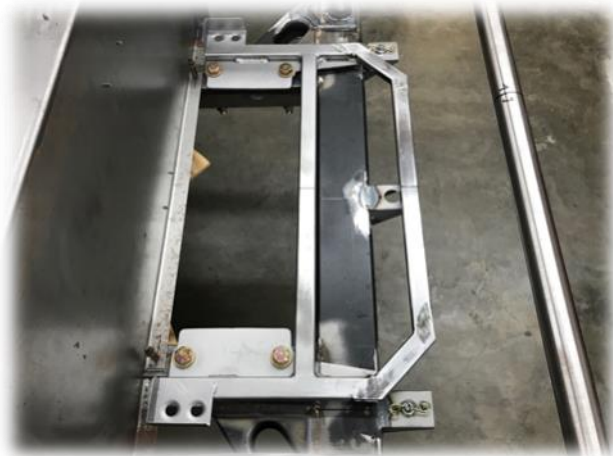
Fuel tank mounting support bracket.
