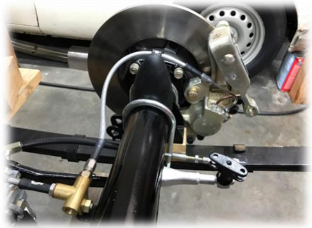
Rear Disc brake set up. Bret's idea to aid servicing.
