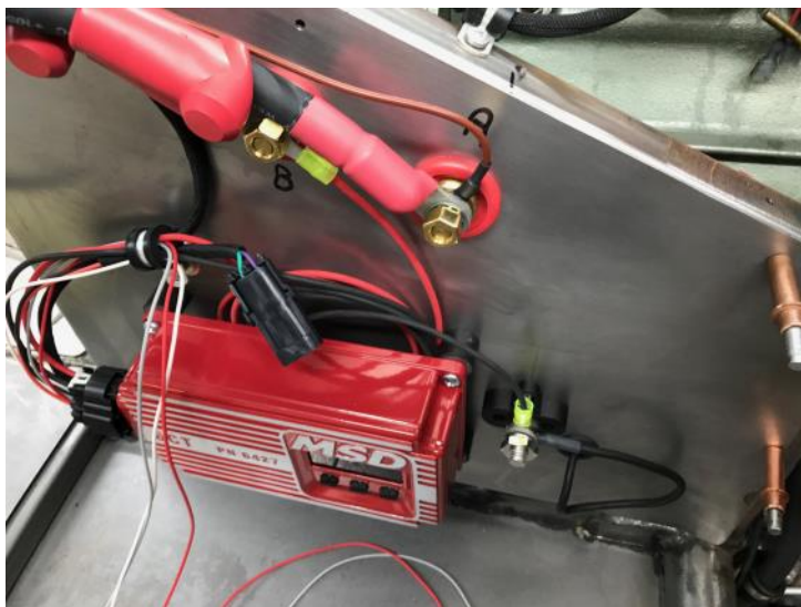
The Devin Healey get's a NEW Electronic Ignition
